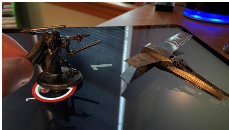
Figure 14. The pewter figure is easily sensed while the steel one isn't [Source: Author].
