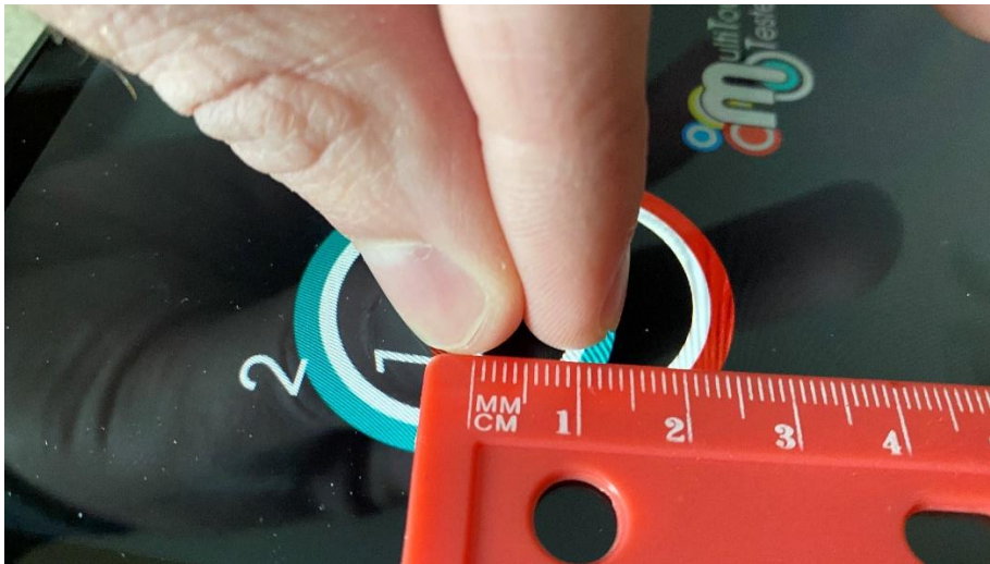
Figure 7. Average tablets need at least 1cm between separate touches [Source: Author].
