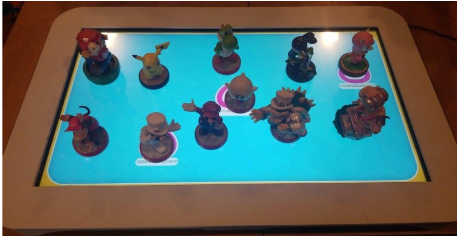
Figure 6. The PlayTable becomes inaccurate as more game pieces are used [Source].
