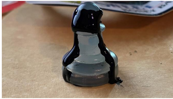
Figure 18. A Chess pawn covered with conductive ink used during Roll [Source: Author].
